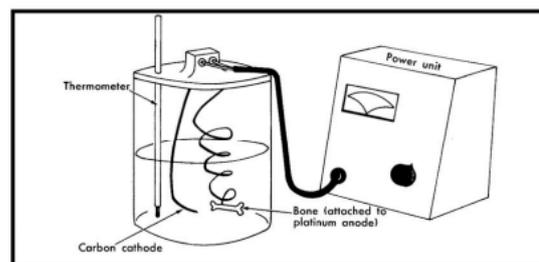
Figure 2: Electrolytic decalcification apparatus
