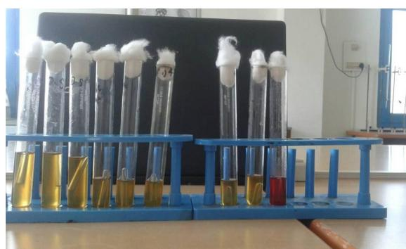
**Figure 5:** Result for MPN after 48 hours
