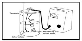
Figure 2: Electrolytic decalcification apparatus
