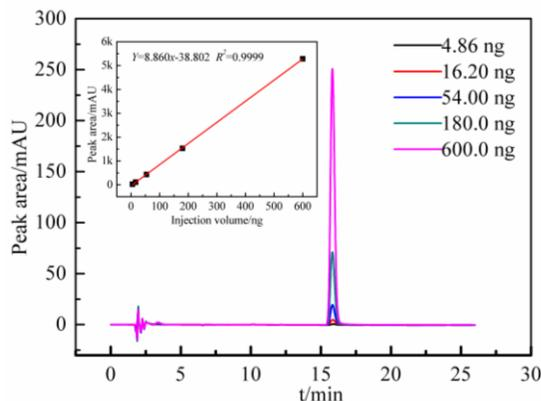
**Fig 6: Plot of peak area versus concentration of reference solutions**
