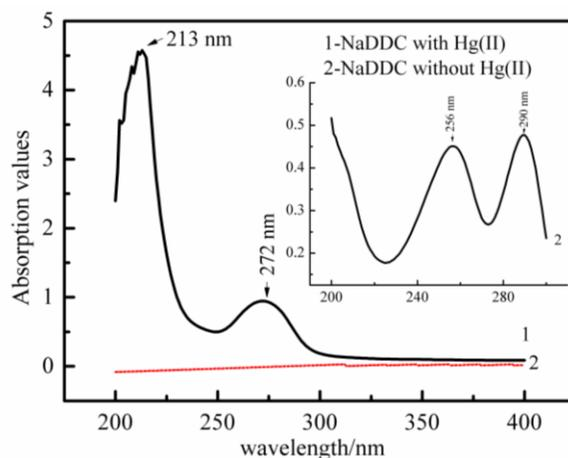
Fig. 3: UV spectrum of Hg(DDC)<sub>2</sub> chelates
