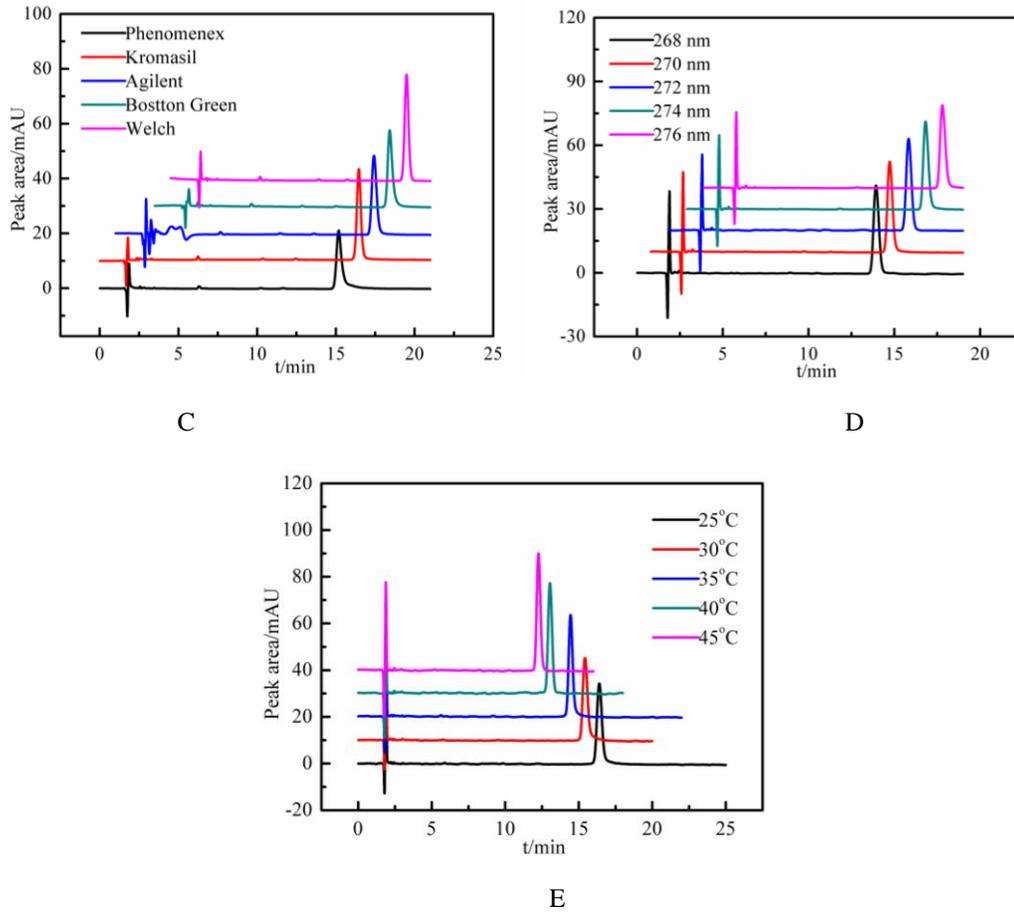
**Fig 4: Chromatograms of robustness: (A) proportion of different mobile phase; (B) various flow rates; (C) different columns; (D) different wavelengths ;(E) different column temperatures**
