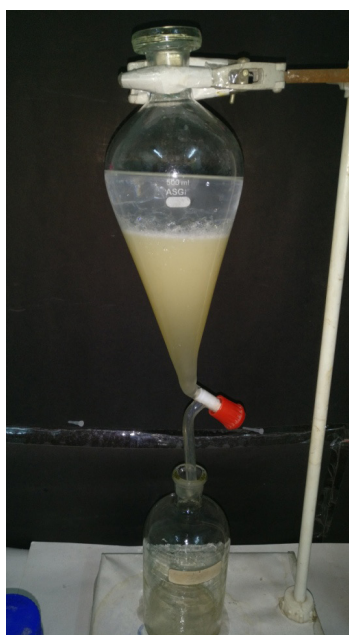
Figure 11: Solvent extraction method
